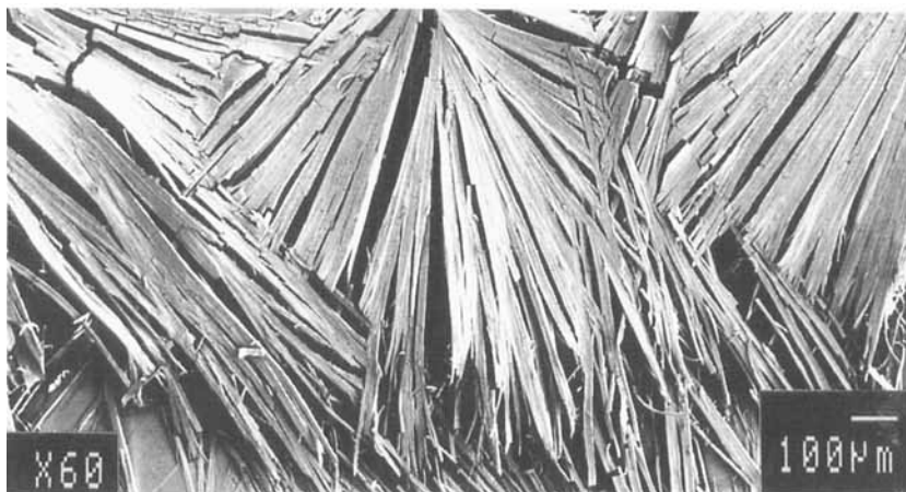
FIGURE 4 SEM microphotograph of \text{HfCl}_2(\text{OH})_2 \cdot 7\text{H}_2\text{O} crystals
